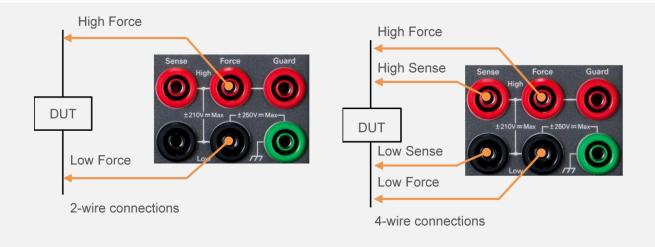
Low current measurements (< 1 nA) require guarding to prevent leakage through the measurement cable. The schematic shown below provides a simplified overview of the guarding technique. Guarded measurements require the use of triaxial cables. A follower (x1) buffer amplifier keeps the guard conductor at the same potential as the center conductor. Since there is no voltage difference, no current can flow from the center conductor to the guard.
